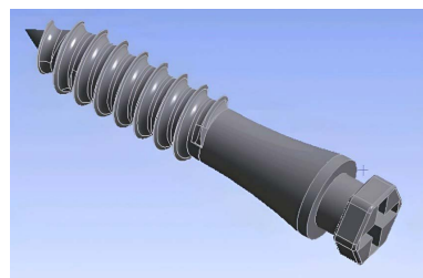
Figure 3. Three-dimensional model of the orthodontic miniscrew (12 × 2 mm JS screw DualTop, Jeil Medical Corporation, Seoul, Korea)—model rendered in Solidworks 2018
