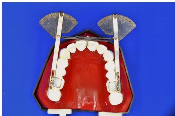
Figure 2. The inclinometer can be used on the stone models and in the oral cavity.
