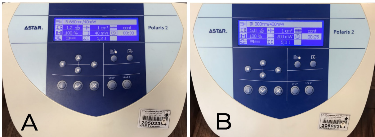
Figure 2. Laser instrument calibration. A. 660 nm beam. B. 808 nm beam.
